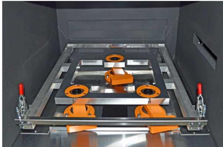
A shaking culture machine is used as the drive unit to make the vortex..
